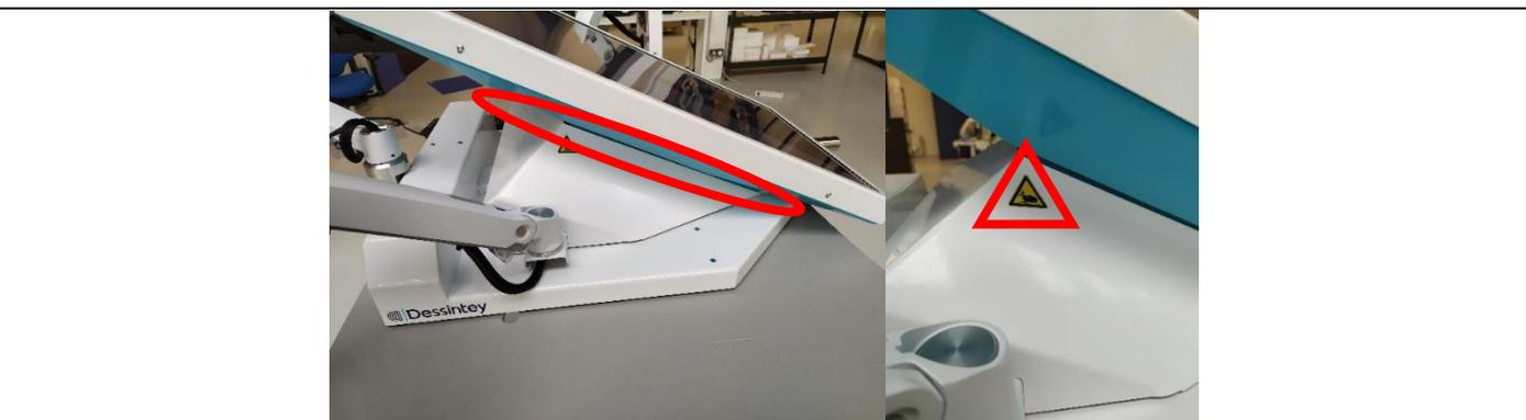
Finger can be trapped with the slot between the column and the table's support
